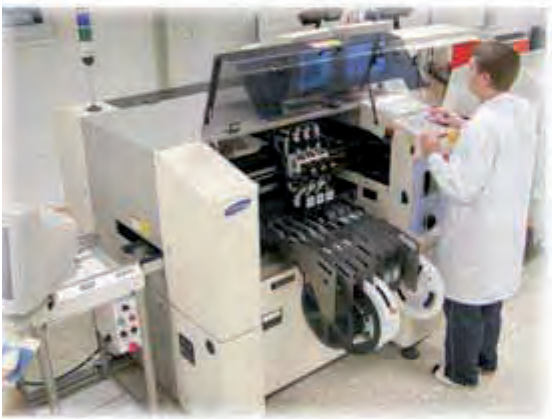
3) SMD components are mounted by pick-up machines. Three heads with laser alignment can place up to 15,000 components an hour. This machine replaces approximately 100 workers.
