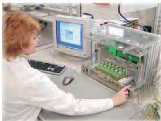
9) After necessary semi-product testing on pin-testers final assembling into enclosures is executed. The actual state of completion is monitored by bar codes during the whole production process.
