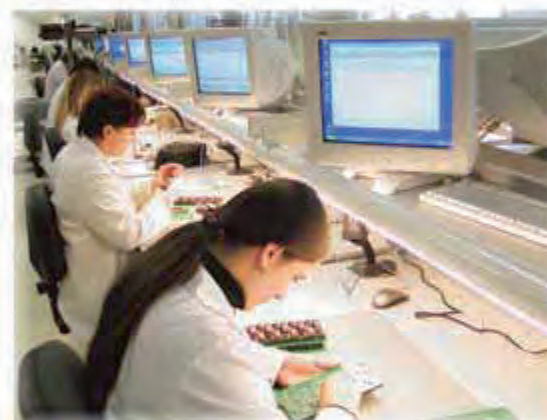
9) After necessary semi-product testing on pin-testers final assembling into enclosures is executed. The actual state of completion is monitored by bar codes during the whole production process.
