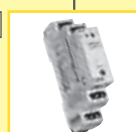
TER-7 Monitoring heating of motor winding in range given by resistance of in-built PTC thermistor (1.8-3.3 kΩ), additional function (memory, reset), output contact 2x8A changeover/ SPDT, supply: AC/ DC 24-240 V.
