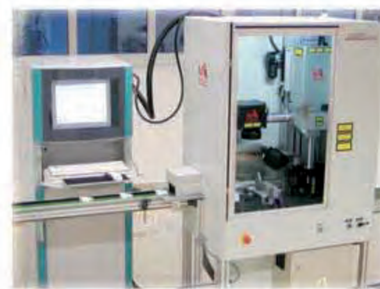
12) In the end the products are fully printed by laser technology. Laser can burn from upper part ( side of the product) and side part ( front panel and terminals) printing one piece takes about 30 s.
