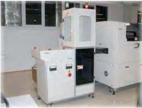
1) Printed circuit boards are placed into a cartridge and then automatically delivered to SMD production line.
