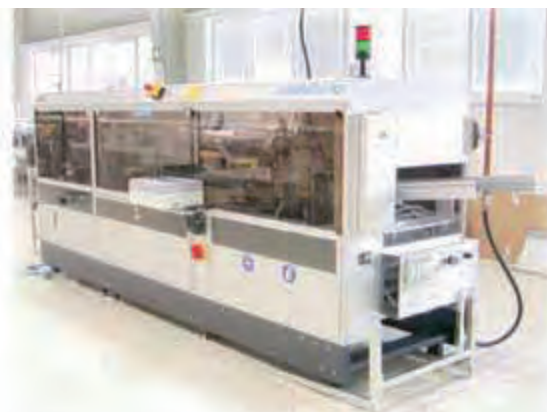
8) Manual placing of classical components is followed by soldering in soldering unit SEHO 8135-PCS which already supports "lead free" soldering technology. Thanks to IR pre-heating, this soldering unit allows operations on PCB together with temperature sensitive components on the upper side of PCB. Soldering unit is equipped by LW soldering jet and Delta jet. These jets allow a good quality.
