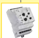
TER-4 Wide and accurate range of setting -40 °C to +110 °C (-40 °F to 230 °F) in ten ranges in one device, fine temperature setting. 2 inputs for NTC sensor, 2 outputs 16 A changeover/ SPDT, additional function (memory, hysteresis, indication of faulty sensor). Supply: AC 230 V or AC/DC 24 V (galv. separated).
