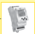
TER-9 Digital multifunction thermostat 2 temperature inputs, 2 outputs 8A changeover/ SPDT, 6 functions, in-built time switch clock, LCD with back light, galvanically sep. supply voltage AC 230 V, 2 MODUL. Temperature range: -40 °C to +110 °C / -40 °C to 230 °F
