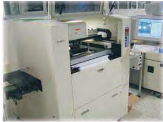
2) Fully automatic adhesive and flux printer distributes adhesive or flux through profile form to the place where the SMD components are then mounted. Part of this process is also 3D optic inspection of the executed operation.
