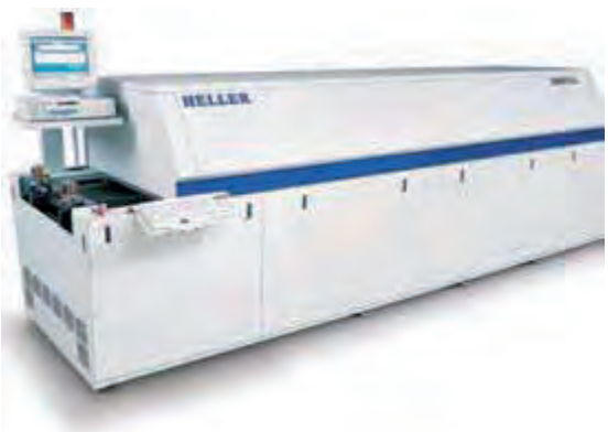
5) Hot-air furnace ERSA serves for glue hardening or to activation of soldering flux by re-melting. The furnace has 3 zones. temperature after curing on 3rd ) output) zone approx. 1400C. For flux re-melting , the starting temperature is 130 °C, middle 180 °C and output is 280 °C.
